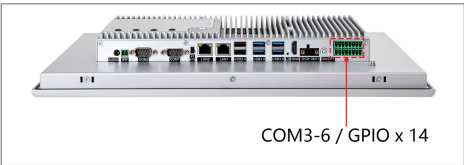
Optional I/O View : iDOOR-4x COM / 14xGPIO
